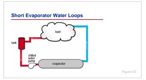
Short water loops may be unavoidable in close-coupled or very small applications, particularly in systems where the load consists of only a few air handlers or processes.
